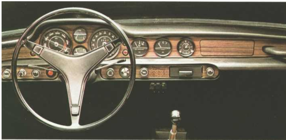
Instrumentation (including the standard tachometer) and dashboard layout in the 1800E and
