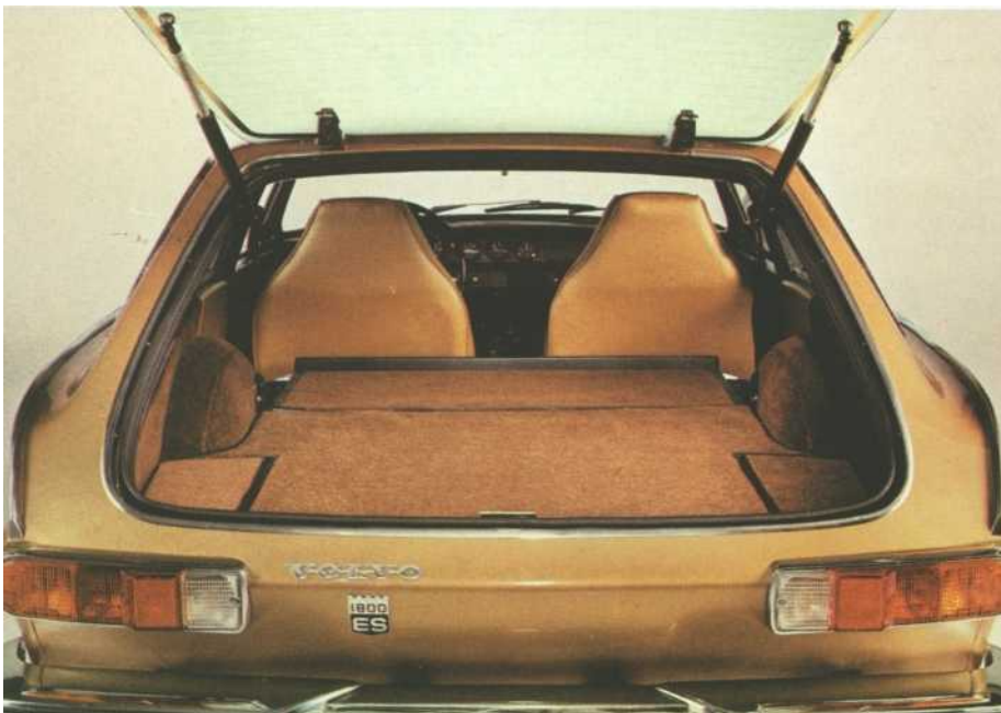
The 1800ES rear window/tailgate opens up a carpeted luggage area 59.8 inches long by 49.2 inches wide by 22.4 inches high.
