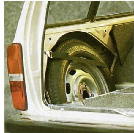
One of two spare wheel wells.
