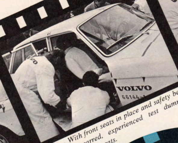
3:49 - Vehicle 66144S - 21 has its front doors removed so cameras can record what happens during the crash. Struts are used to compensate for the missing doors.
