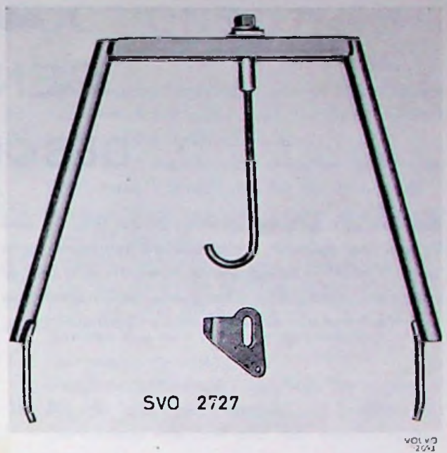
Fig. 3. Tool for removing oil sump, 140-series
