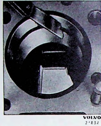
Fig. 32. Measuring the piston ring gap
