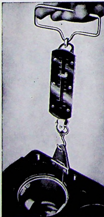
Fig. 31. Checking the piston clearance
