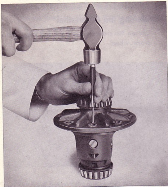
Fig. 33. Removing lock pin
