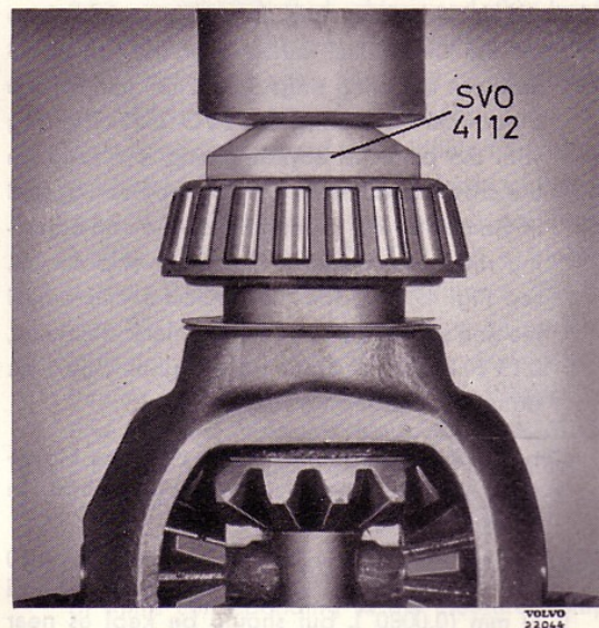
Fig. 54. Fitting the differential carrier bearing
