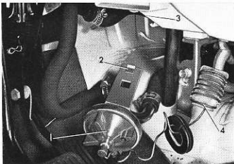
Fig. 8-79. Replacing heater control valve
