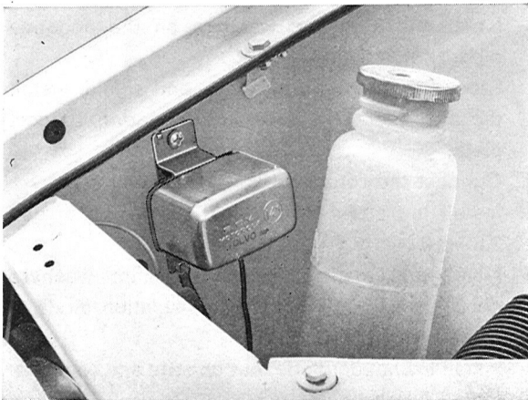
Fig. 3-20. Voltage regulator installed
