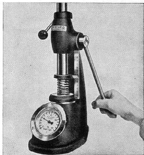
Fig. 25. Testing the springs
