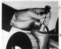
Fig. 19. Checking the oil level
