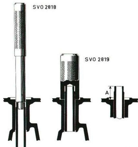
Fig. 2-33. Replacing valve guides
