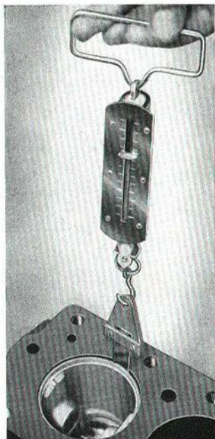
Fig. 2-37. Measuring piston clearance
