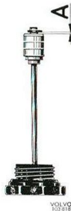
Fig. 2-125. Damper plunger clearance
