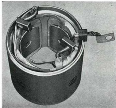
Fig. 3-91. Stator with soldered brushes
