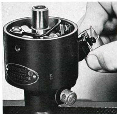
Fig. 3-102. Removing primary connection
