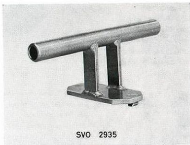
Fig. 3-149. Special tool for removing and installing tank fittings
