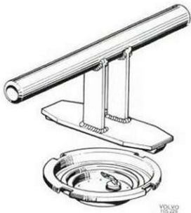
Fig. 3-164. Tool for removing sender for fuel gauge
