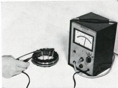
Fig. 3-61. Checking stator resistance
