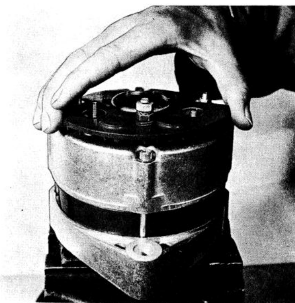
Fig. 3-6. Removing the isolation diodes
