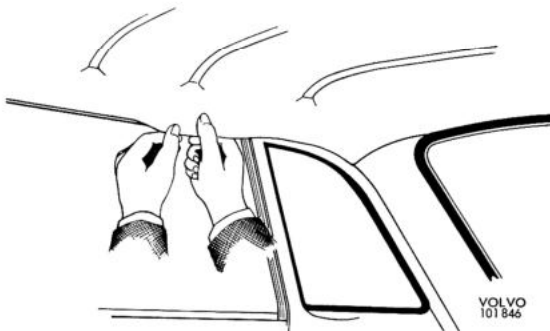
Fig. 8-32. Removing the headlining
