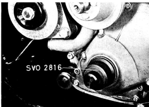
Fig. 2-31. Fitting oil seal
