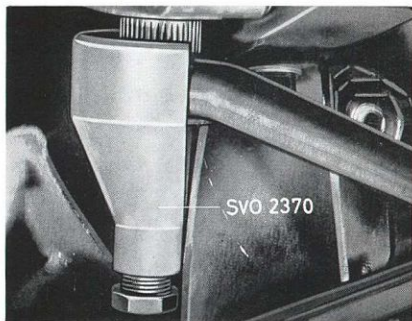
Fig. 6-54. Removing pitman arm
