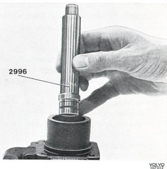
Fig. 6-107. Fitting needle bearing
