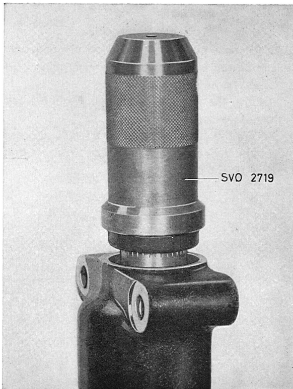
Fig. 6-61. Fitting sealing ring, pitman arm shaft
