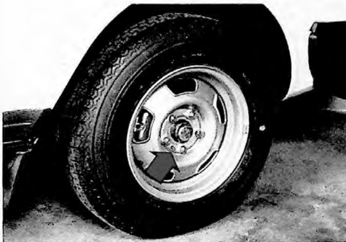
Stud fits into small hole in rim
