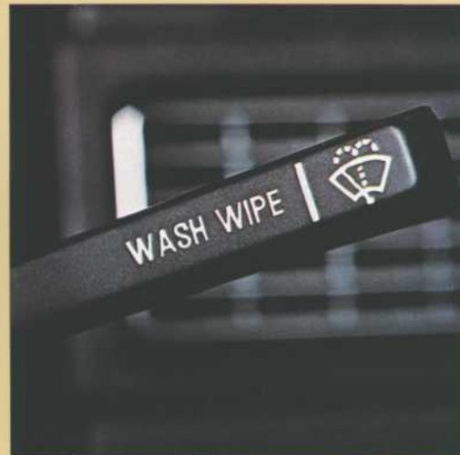
The windscreen wipe/wash stalk has a special position for intermittent windscreen wiper operation during drizzle.
