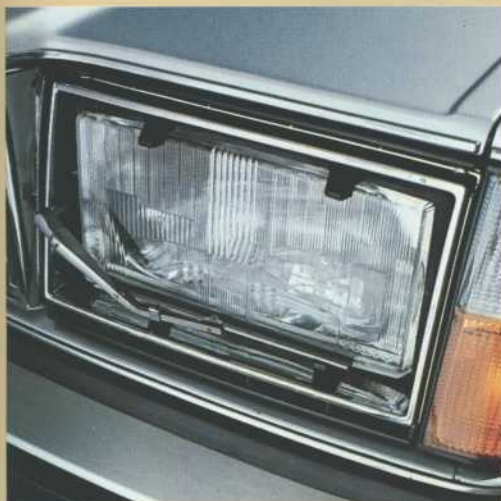
The large rectangular halogen headlights have separate reflectors for full and dipped beams to ensure the best visibility at all times. Washers and wipers keep the headlight glass clean from dirt.
