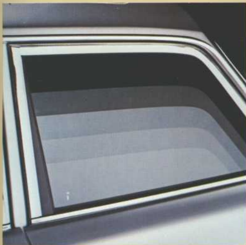
GLE models have electrically operated windows in both front and rear doors. The rear windows can be locked from the driving seat. All windows have tinted glass.
