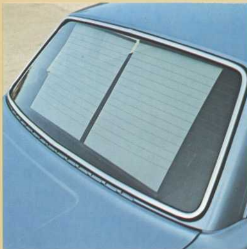
The rear window is electrically heated for rapid defrosting. The 264GLE also has a two part blind to protect rear seat passengers from intensive sunshine without obstructing the view of the driver.
