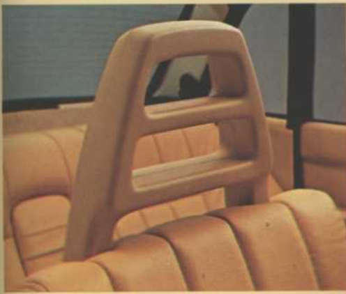
Volvo 264 and 265 cars have integral head restraints. The 264GLE also has head restraints on the rear seats.
