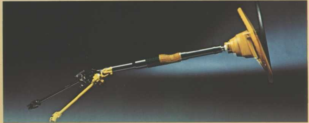
The steering wheel and steering shaft are designed to provide maximum safety in the event of a collision: The lower steering shaft section 'gives' way, the steering shaft 'telescopes', the steering
