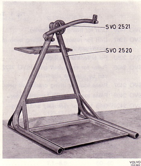
Fig. 5 Stand SVO 2520 and fixture SVO 2521 for engine
