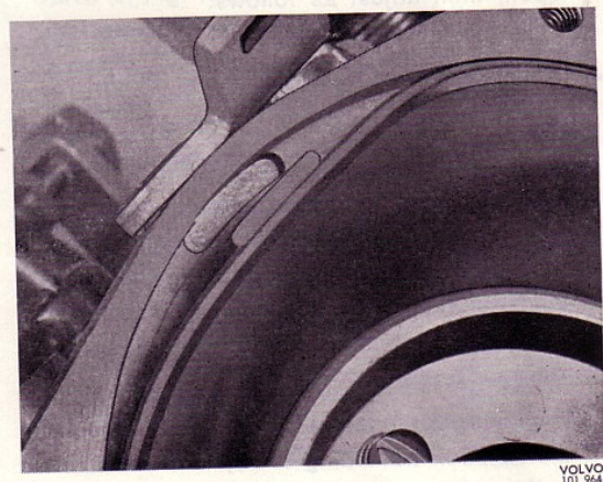
Fig. 104 Diaphragm in carburettor housing
