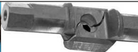
Unexpected find on rebuild. One of the two cross shafts had cracked through. Spider gears run either side of the shaft(s). Cross shafts are the most common
