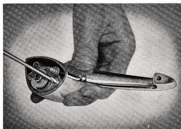
Fig. 15. Dismantling the lock handle.
