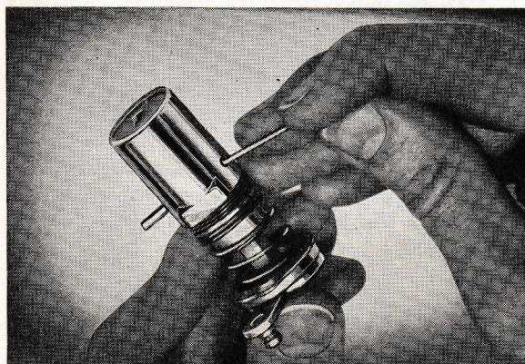
Fig. 16. Pressing out the lock peg.
