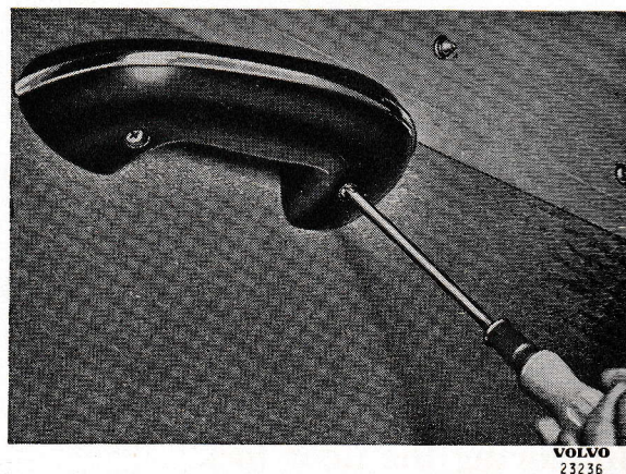
Fig. 8. Removing the armrest.
