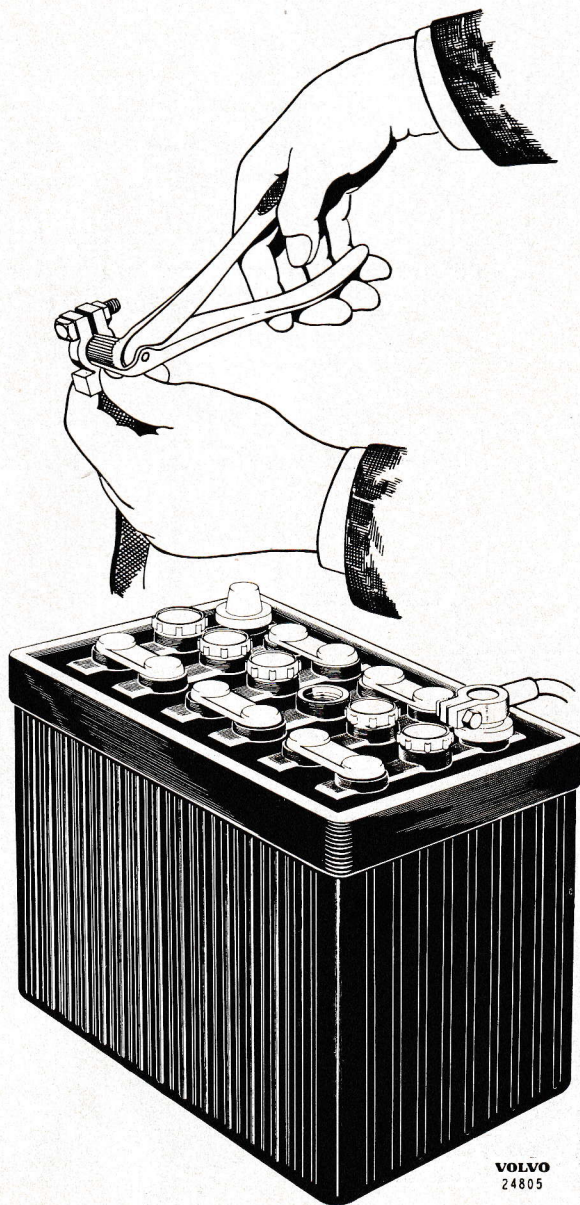
Fig. 13. Cleaning battery cable terminal.
