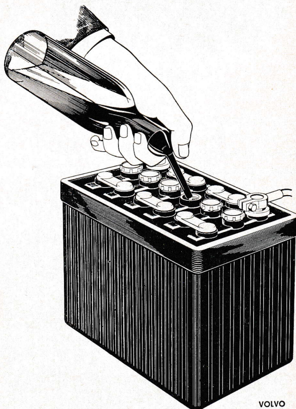
Fig. 10. Topping-up with distilled water.
