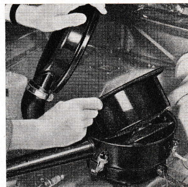
Fig. 16. Disassembling the air cleaner (B 18 B, B 18 D).
