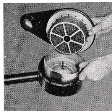
Fig. 17. Disassembling the air cleaner (B 18 A, B 16 A).
