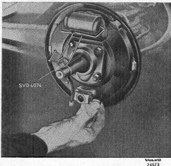
Fig. 44. Removing the adjusting plunger.
