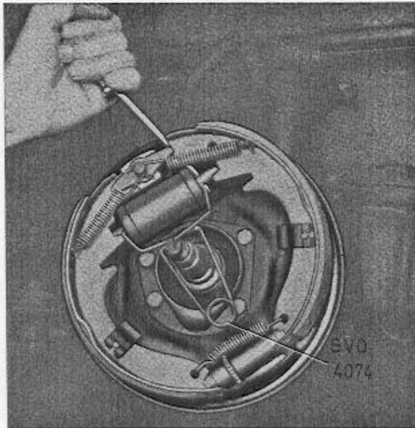
Fig. 53. Removing the wheel unit cylinder.
