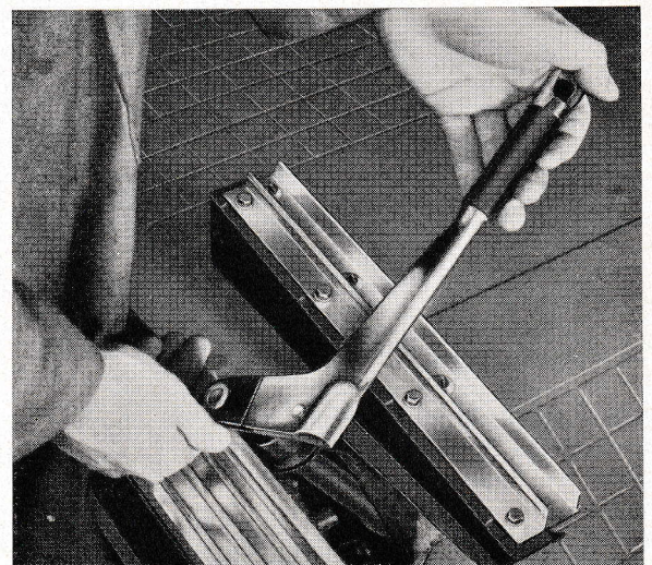
Fig. 60. Removing the handbrake lever.
