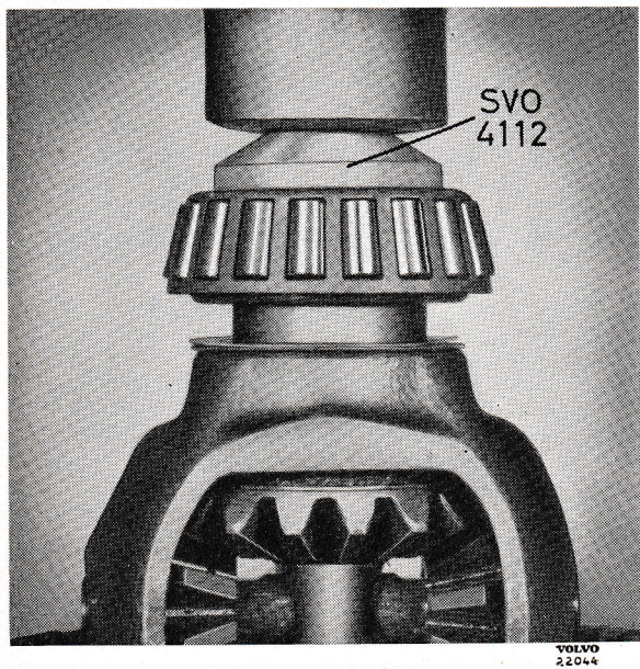
Fig. 30. Fitting the differential carrier bearing.
