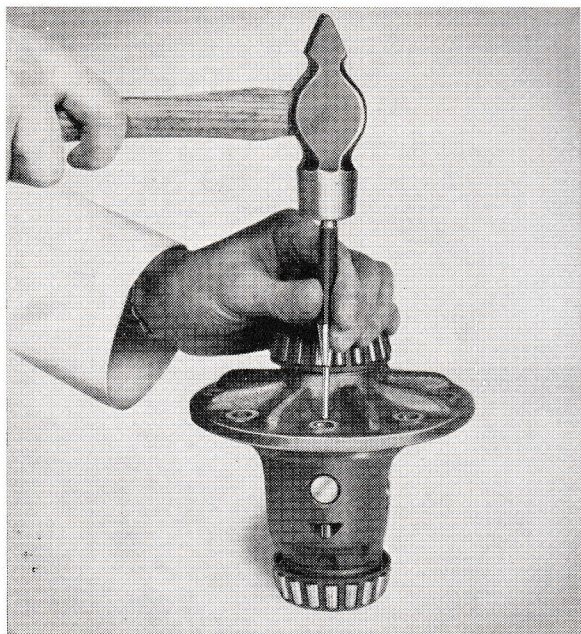
Fig. 12. Removing the lock pin.
