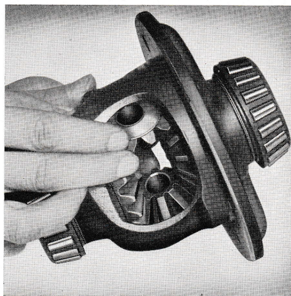
Fig. 28. Fitting the differential pinion gears.
