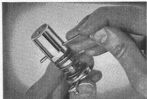
Fig. 16. Pressing out the lock peg.
