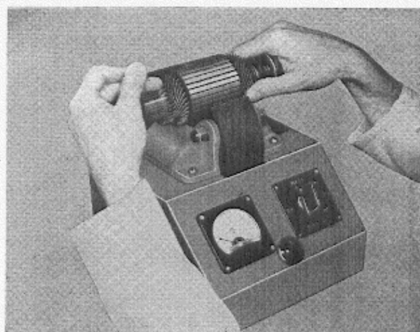
Fig. 24. Testing the rotor.
