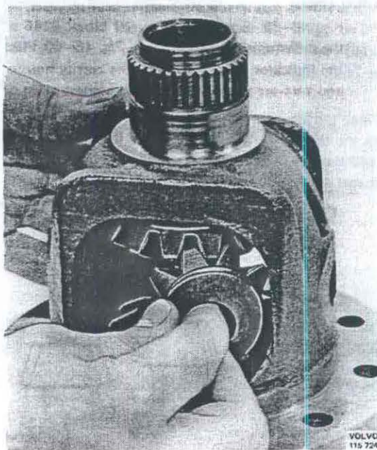
Fig. 46-52. Fitting the diff. side gears
