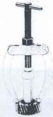
Fig 46-141 Removing the races
