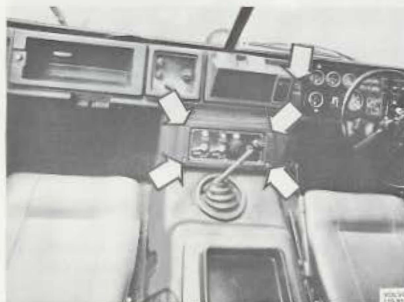
Fig. 26-7. Removing the cover over the radiator and the panel for the diff. lock controls
