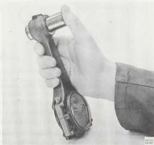
Fig. 21-30. Gudgeon pin fit
