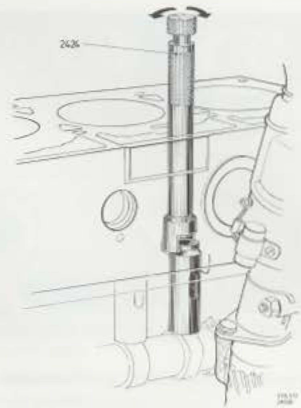
Fig. 21-19. Removing and installing valve tappets
