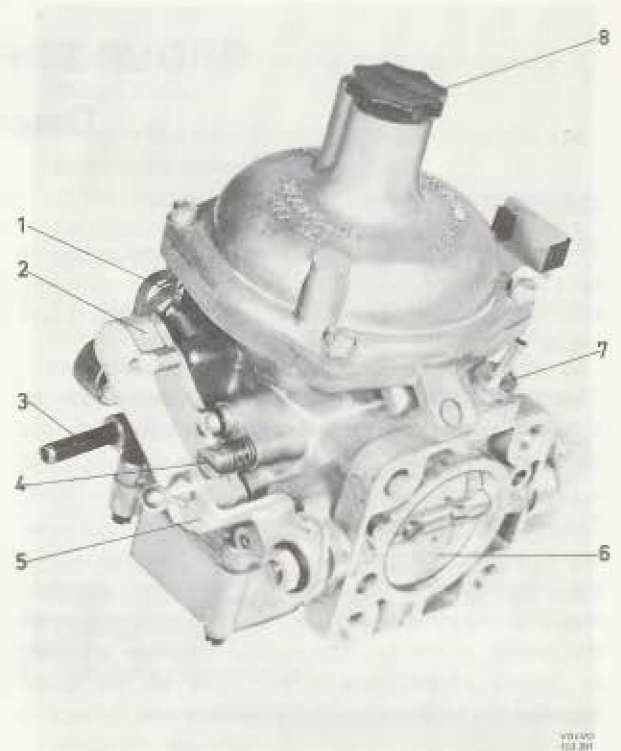
Fig. 23-4. Rear carburettor, from right
