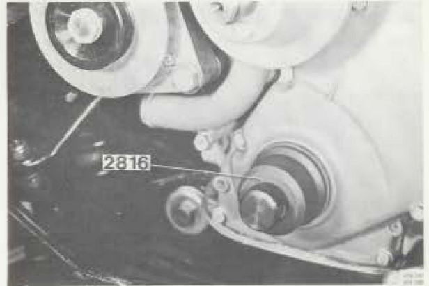
Fig. 21-36. Installing the timing gear casing seal
