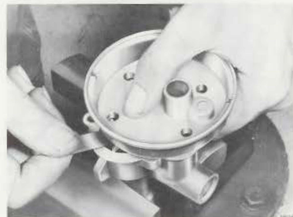
Fig. 22-7. Measuring the axial clearance
