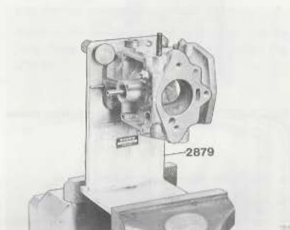
Fig. 21-31. Mounting carburettor on fixture 2879
