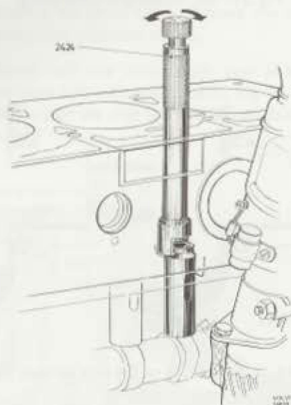
Fig. 21-45. Lifting out valve tappets
