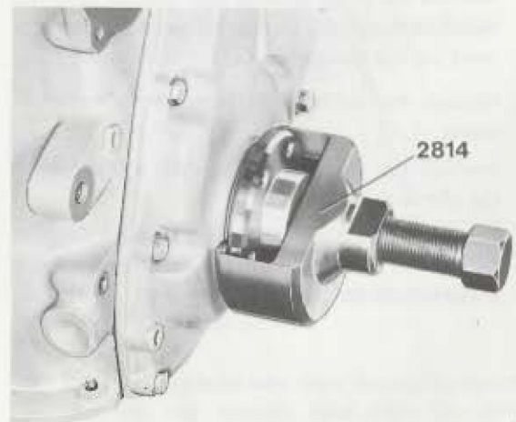
Fig. 21-8. Removing the polygon hub
