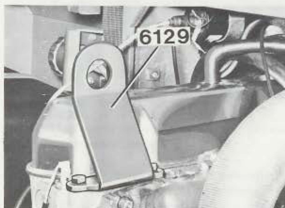
Fig. 21-5. Attaching the lifting lug 6129
