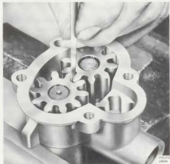
Fig. 22-6. Measuring the backlash
