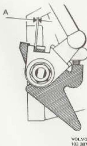
Fig. 27-2. Adjusting throttle control, idle position A = 0.1 mm (0.0039'')
