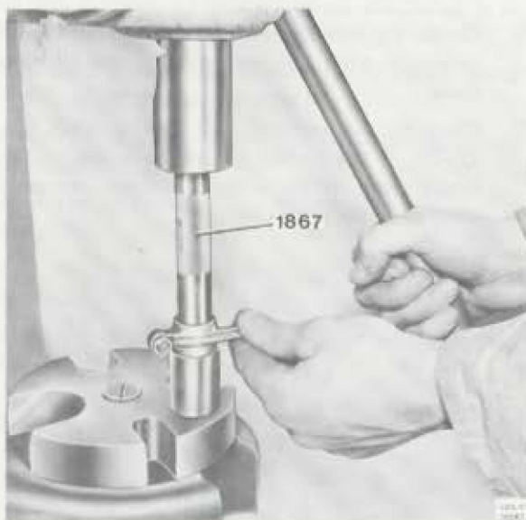
Fig. 21-24. Replacing a rocker arm bushing
