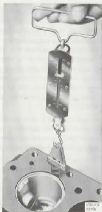
Fig. 21-27. Measuring the piston clearance
