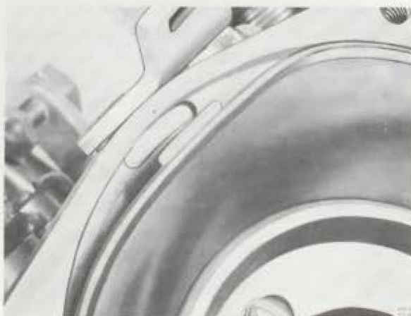
Fig. 23-25. Diaphragm in carburettor housing
