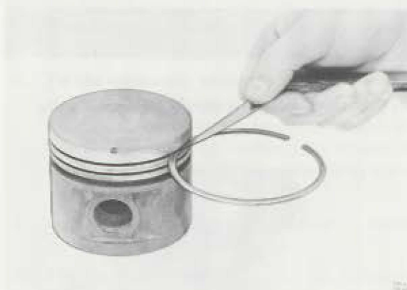
Fig. 21-28. Measuring the piston ring clearance in groove
