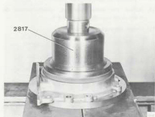
Fig. 21-47. Pressing in sealing ring
