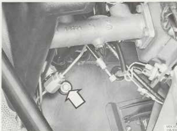
Fig. 26-8. Retaining bolt on side of radiator
