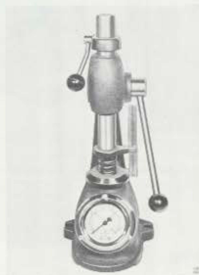
Fig. 21-23. Testing a valve spring
