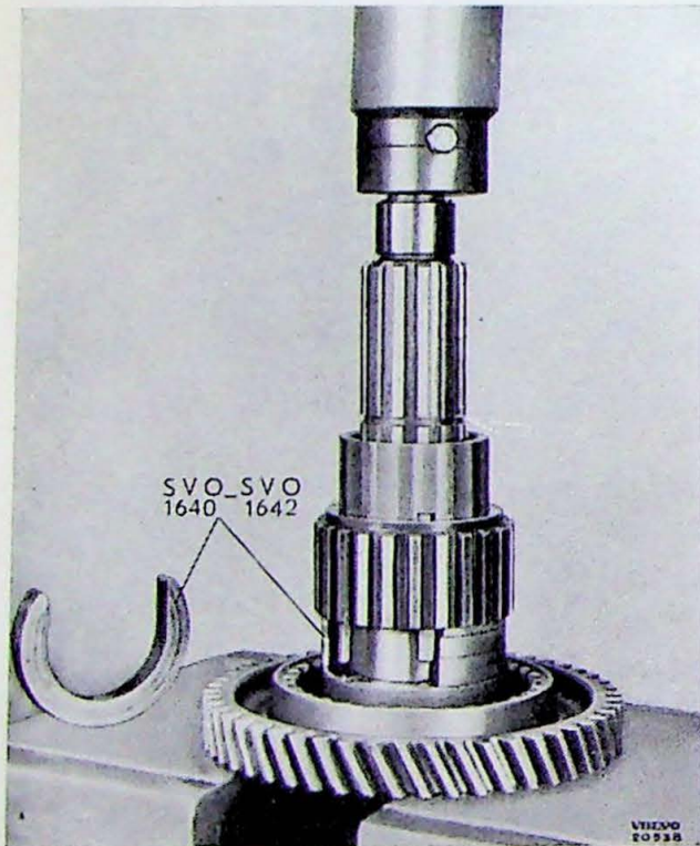
Fig. 3—18. Removing the synchronizing device hub from the mainshaft.
