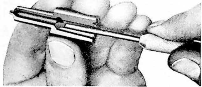
21238 Fig. 1—124. Cleaning walls of pressure chamber.
