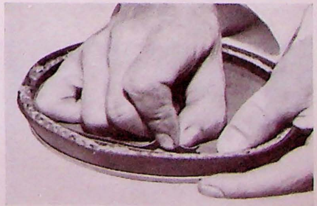
Fig. 7—37. Assembling the vacuum plunger.
