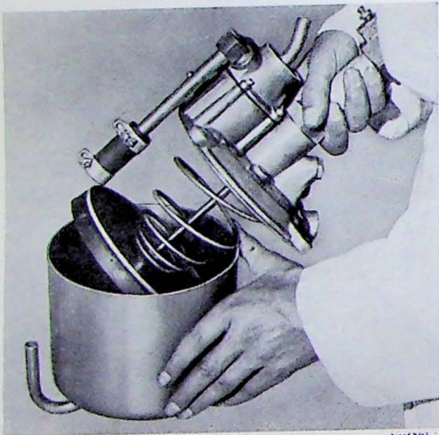
Fig. 7—39. Assembling the Hydrovac.
