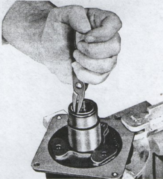
Fig. 34. Removing Seal Seat Retaining Snap Ring
