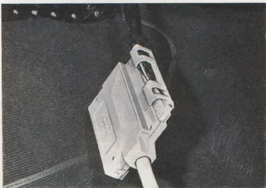
Fig. 2—35. Test instrument connected to the cable harness
