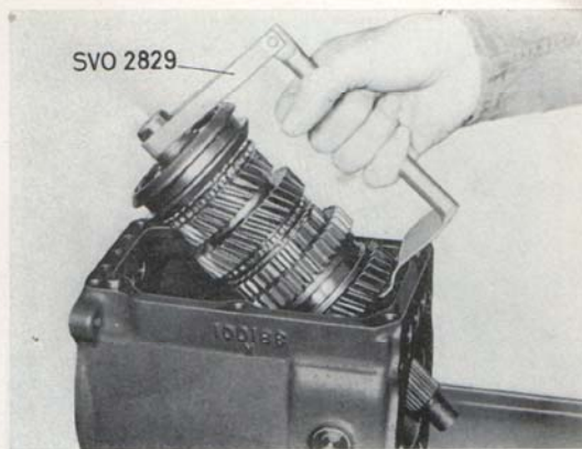
Fig. 4-7. Lifting out the mainshaft
