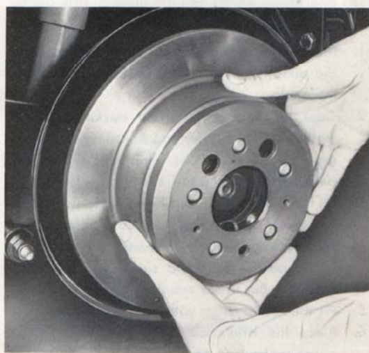
Fig. 5-17. Removing the brake drum
