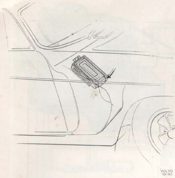
Fig. 2—6. Control unit, mounted
