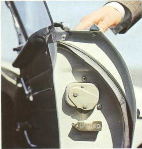
The patented safety door latch keeps doors closed even under severe impact.
