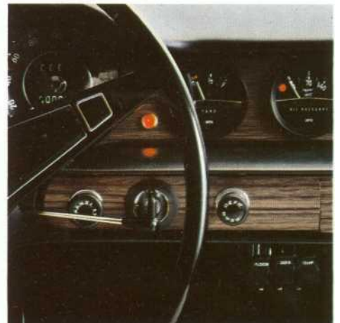
One more speed. Electric overdrive lets the 1800E go faster while the engine goes slower. Just flick the lever.
