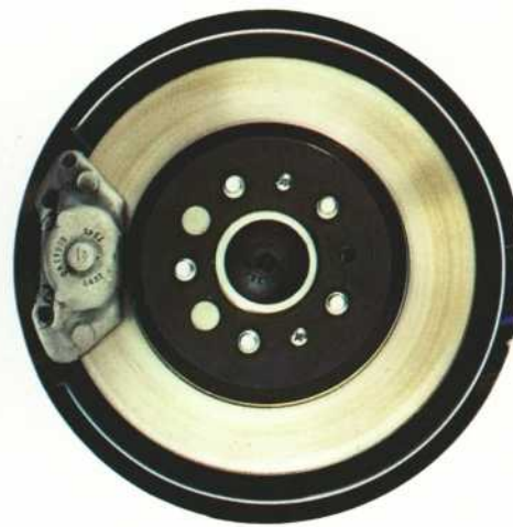
Power assisted disc brakes on all four wheels. Sure stopping, low pedal loads.
