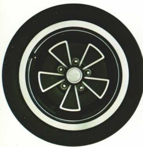
5" steel rims. Cast aluminium "mag" type hubs. 165 HR 15 radial ply tyres.
