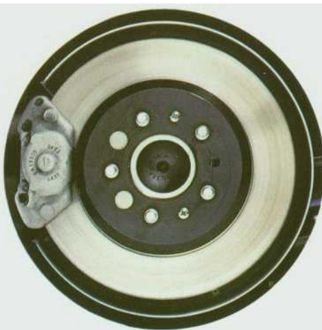
Disc brakes on all four wheels. 83-square inches of pad area and power assist too.
