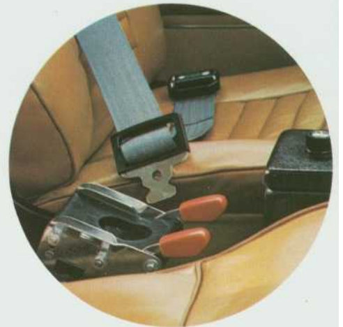
The front seats have factory-fitted three-point safety belts. Convenient snap-action locks.
