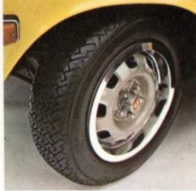
Low profile radial ply tires are standard equipment on all live wheels.
