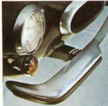
But new bumpers aren't designed to bump but rather, to take a bumping. They're mounted on oil-filled, hydraulic shock absorbers and designed to take impacts at 5 mph (front) and 2.5 mph (rear).
