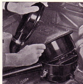
Fig. 22. Dismantling the air cleaner (B 16 B, B 18 D)
