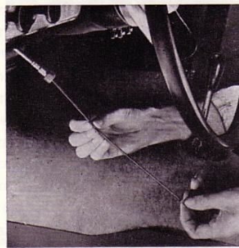
Fig. 28. Lubricating the drive cable
