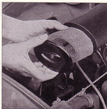
Fig. 15. Removing the air cleaner element (B 16 A)
