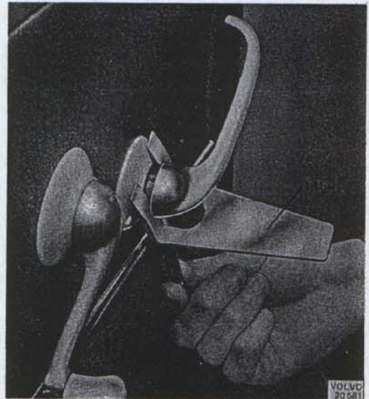
SVO 1460 Holder for removing door handle and window winder.
