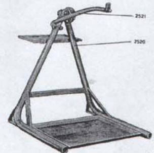
SVO 2920 Stand with engine fixture SVO 2521. Used when reconditioning engine.
