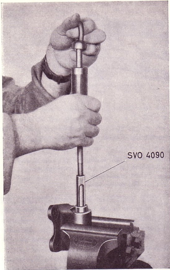
Fig. 44. Removing needle bearing. VOLVO 23750
