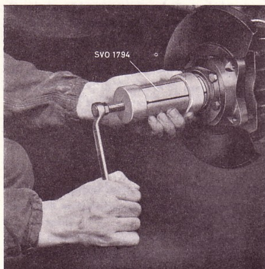
Fig. 18. Removing the inner bearing.
