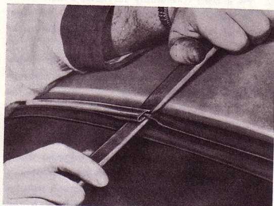
Fig. 34. Removing trim moulding from rubber strip.
