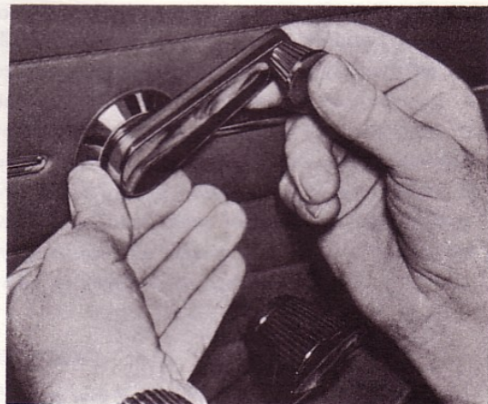
Fig. 7. Removing winding handle, late prod.
