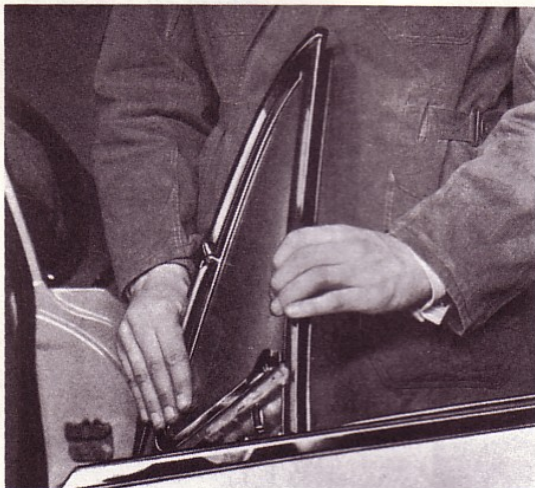
Fig. 20. Taking out the ventilation window with frame.
