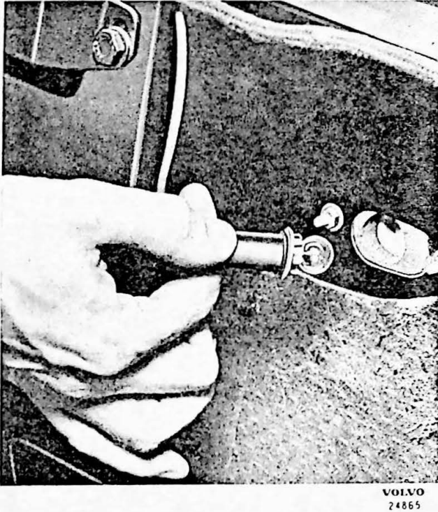
Fig. 10-67. Number plate light, removing the bulb
