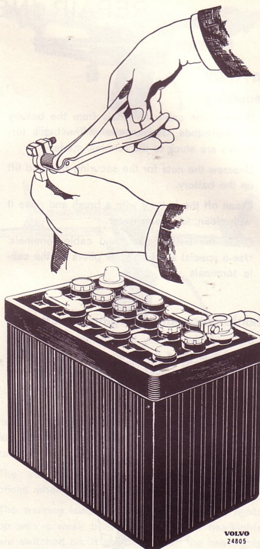
Fig. 17. Cleaning battery cable terminal
