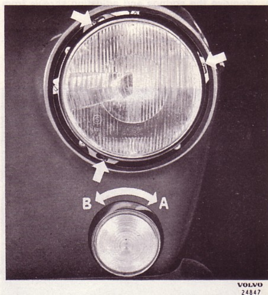
Fig. 80. Removing the headlamp insert retaining ring and flasher and parking lamp
