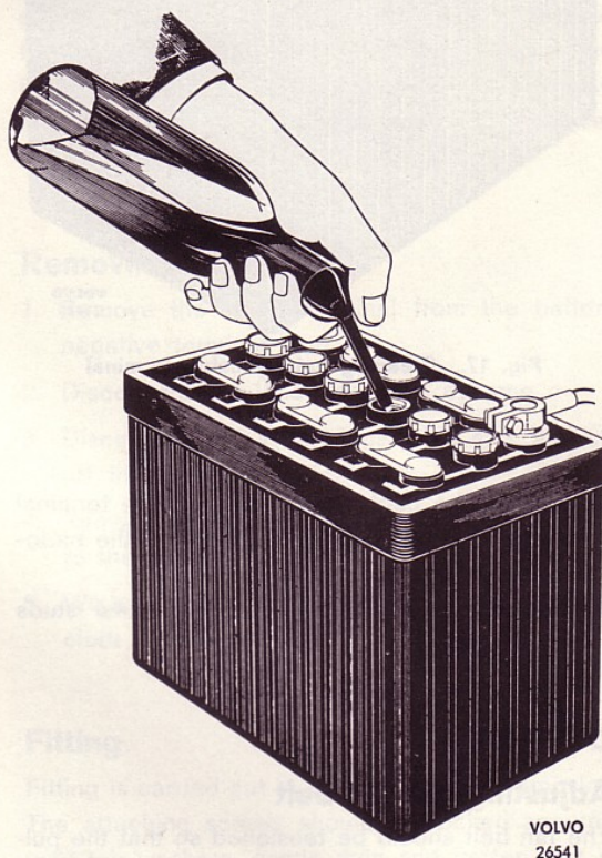
Fig. 14. Topping-up with distilled water
