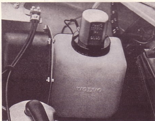
Fig. 103. Windscreen washer, late prod., fitted
