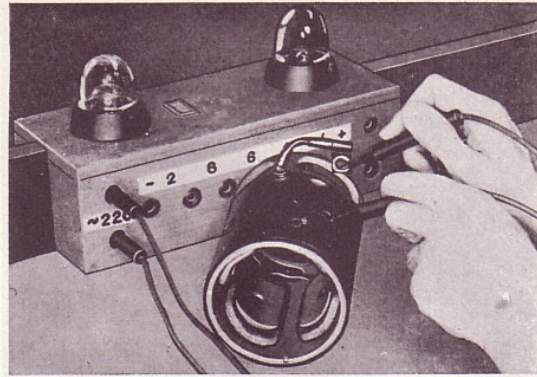
Fig. 59. Testing the field winding
