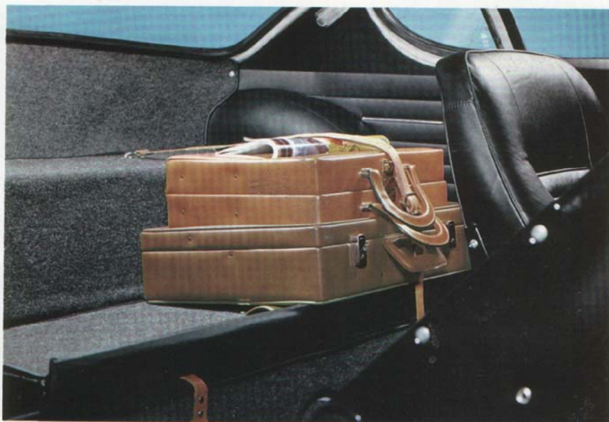
When folded down, the occasional seat provides an extra and roomy platform for luggage.
