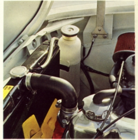
The sealed cooling system keeps the radiator from blowing its stack.
