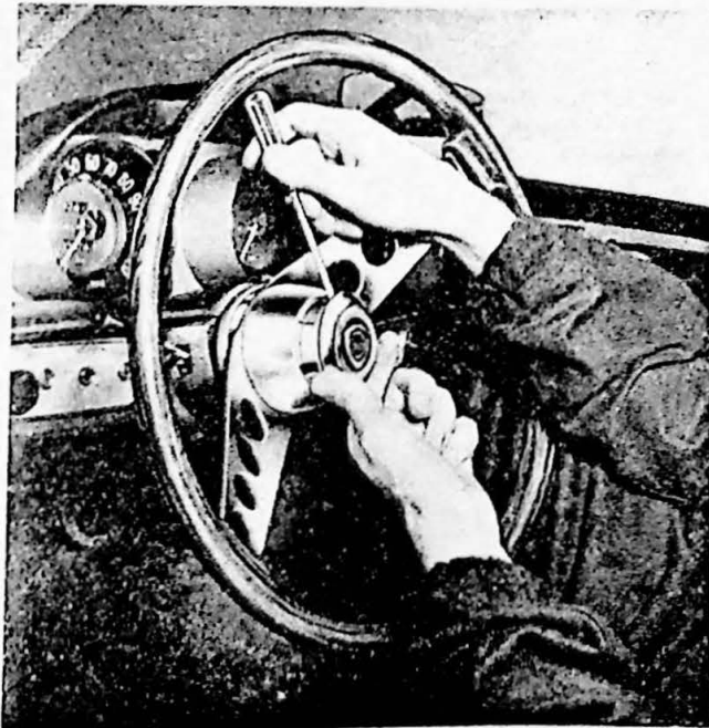
Fig. 6-19. Removing the horn button
