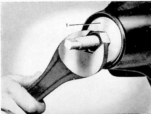
Fig. 17. Fitting bearing rings. 1. Press tool SVO 4047.
